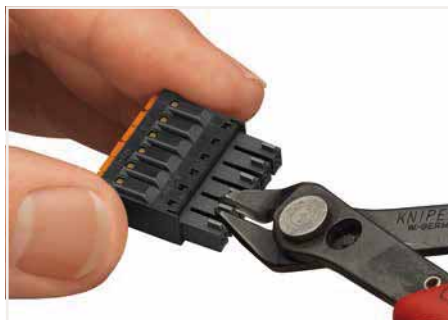
Coding a female connector – removing coding finger(s).
