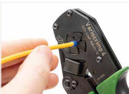
Squeeze handles until ratchet mechanism is released.
