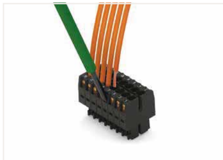
Inserting a conductor via (2.5 x 0.4) mm screwdriver.
