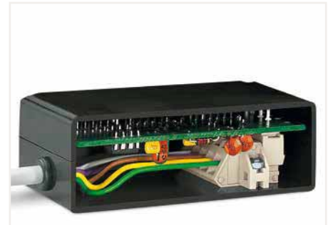
Angled female connector – male header with straight solder pins is used for horizontal PCB mounting in narrow housings.
